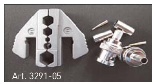
Art. 3291-05 Coaxial RG 58.59.62.6. 6.48 / 5.41 / 2.5 / 1.72 / 8.23 mm 2 0.255 / 0.213 / 0.1 / 0.68 / 0.324"
